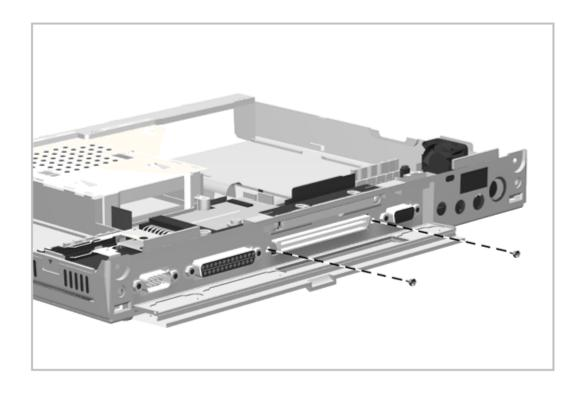
Figure 5-58. Removing the System Board Screwlocks
